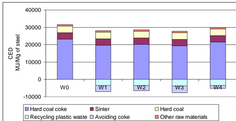
**Fig. 3** Influence of main input factors in blast furnace technology on fossil fuels consumption, per one ton of liquid steel based on CED method (own calculations in the SimaPro)
