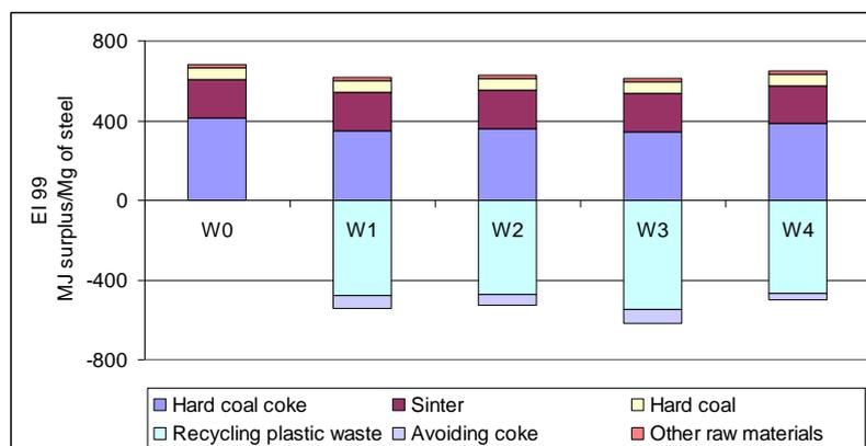
**Fig. 1** Influence of main input factors in blast furnace technology on fossil fuels consumption, per one ton of liquid steel based on EI 99 method (own calculations in the SimaPro)
