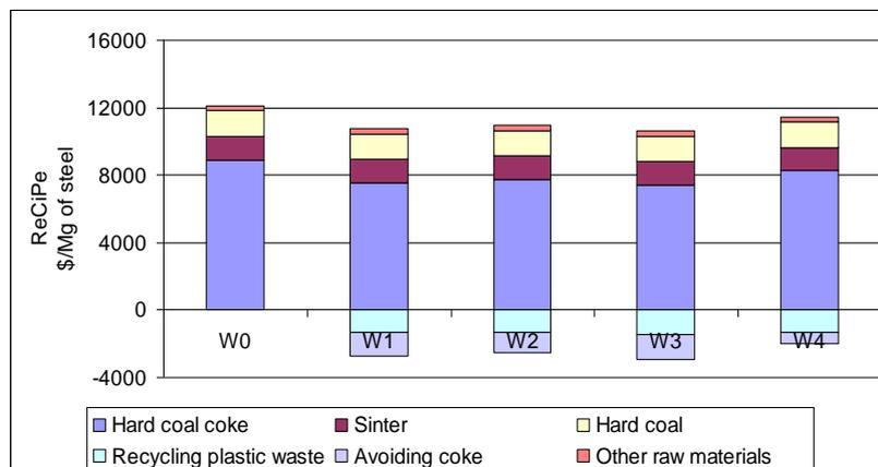
**Fig. 4** Influence of main input factors in blast furnace technology on fossil fuels consumption, per one ton of liquid steel based on ReCiPe method (own calculations in the SimaPro)
