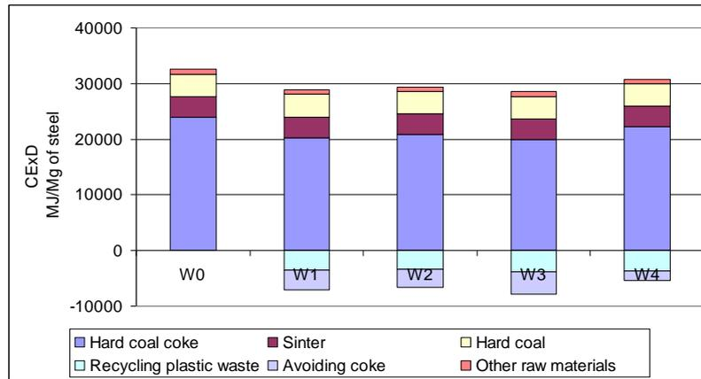
**Fig. 2** Influence of main input factors in blast furnace technology on fossil fuels consumption, per one ton of liquid steel based on CEExD method (own calculations in the SimaPro).
